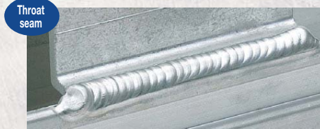
Welding current 130 A, AC frequency 150 Hz, speed 25 cm/min, sheet thickness 3 mm
